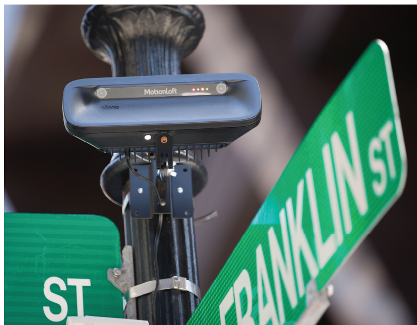
Top: Boston Police Department bicycle officers regularly patrol the Downtown Boston neighborhood. Bottom: Motion-activated street sensors count pedestrians and vehicles 7 days a week, 24 hours a day.
